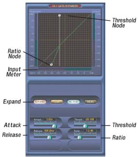
Gate/Expander with Expand on
